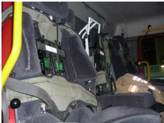
Breathing apparatus is set-up ready in the fire truck to minimise the time needed to be ready to fight a fire
