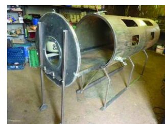
Roger Frank put his engineering background to good use, rolling and welding all the steel components himself.
